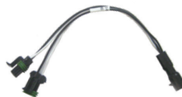
VHMS3007 1 - PACCAR - FEMALE 2 - PACCAR - MALE - FOR CONNECTING FRONT & REAR AIR CLEANER LIGHTS
